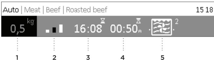
Preset values will appear. Rotate the KNOB and confirm by pressing the KNOB to change these settings.
