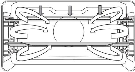
In this operating mode, the grill heater and the fan operate simultaneously. Suitable for grilling meat, fish, and vegetables.
