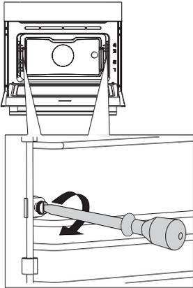
**1** Undo the screw. Use a screwdriver.
