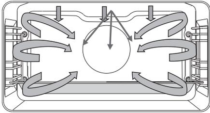
This system uses a combination of microwaves and grill with fan to cut the cooking time.
