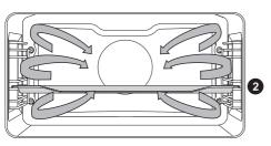
Round heater and the fan will operate. The fan installed in the back wall of the oven cavity makes sure the hot air constantly circulates around the roast or pastry.
