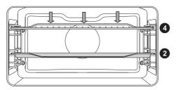
When grilling food with the large grill, the upper heater and the grill heater fitted on the ceiling of the oven cavity will operate.
