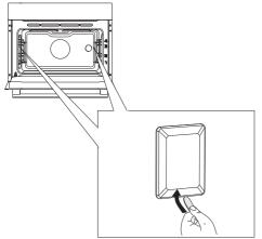
Use a flat screwdriver to release the bulb cover and remove it.
