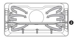
The bottom heater, the round heater, and the hot air fan will operate. Suitable for baking pizzas, apple pies, and fruitcakes.
