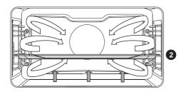
This is used for baking leavened but lowrising pastry and for preserving fruit and vegetables. Use the second guide from the bottom and a rather shallow baking tray to allow the hot air to circulate across the upper side of the dish.
