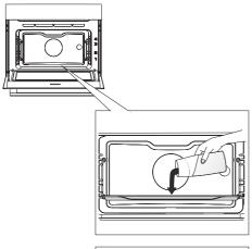
Turn the COOKING SYSTEM SELECTOR KNOB to Aqua Clean. An icon will be displayed along with the PRESET TEMPERATURE and the time of 30 minutes.
