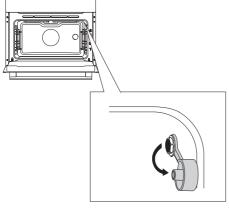
Remove the metal cap (the socket is in the front upper corner of the oven right wall).
