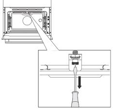
**1** To remove the heater, undo the screw located at the front of the oven cavity ceiling.
