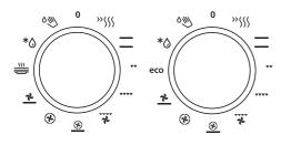
Rotate the knob (left and right) to select 0 COOKING SYSTEM (see program table). The selected icon will appear on the display.
