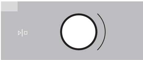
**1** Rotate the SETTINGS KNOB (-/+ ) and first set the minutes; then, the cursor will switch to hours. After three seconds, the settings will be saved.
