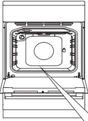
**1** Turn the COOKING SYSTEM SELECTOR KNOB to Aqua Clean. 2. Set the TEMPERATURE KNOB to 70 °C.
