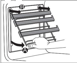
**A** Hold the guides by the bottom side and pull them towards the center of the oven cavity.
