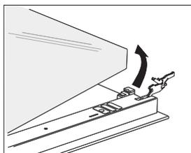
**2** Hold the door glass pane by the lower edge; slightly lift it so that it is no longer attached to the support; and remove it.
