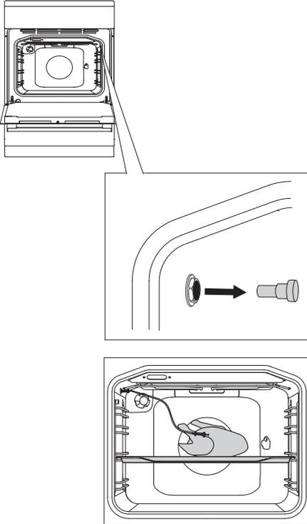
**1** Remove the metal cap (the socket is in the front upper corner of the oven right wall).
