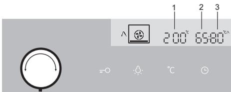
**3** Turn the COOKING SYSTEM SELECTOR KNOB (hot air and lower heater). Symbol, preset temperature, current temperature, and set temperature will appear on the display. If the probe temperature is below 30 °C, the display will read "-- : 80". Press the START key.
