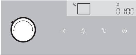
Turn the COOKING SYSTEM SELECTOR KNOB to defrosting. TIME will be displayed. This time setting can be adjusted. Press the START key.
