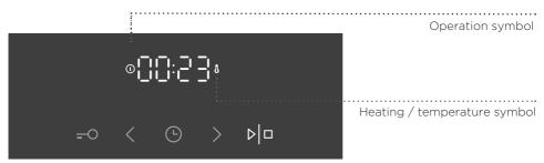
While the oven is heating up, the temperature symbol will flash. When the oven reaches the set temperature, the symbol will light up and a short beep will be sounded.
