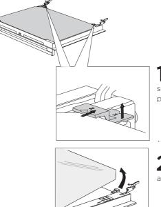
1 Slightly lift the supports on the left and right side of the door (marking 1 on the support) and pull them away from the glass pane (marking 2 on the support).
