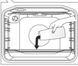
**2** Pour 0.6 I of water into a glass or shallow baking dish and insert it into the lower guide.
