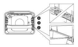
With telescopic extendible guides, first pull out the guides of one level and place the grid or the baking tray onto them. Then, push them in with your hand as far as they will go.
