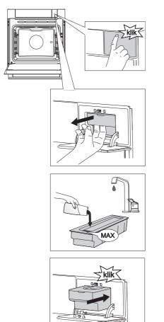
Press on the spot with the sticker to open the tank door.
