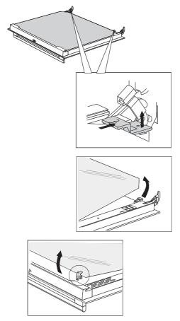
**1** Slightly lift the supports on the left and right side of the door (marking 1 on the support) and pull them away from the glass pane (marking 2 on the support).
