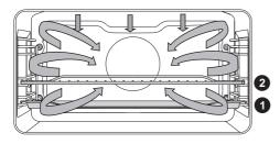
In the Auto Roast mode, the upper heater will operate in combination with the grill heater and the round heater. It is used for roasting all types of meat.
