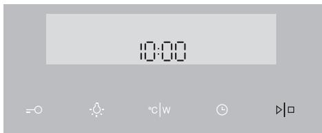
**2** Confirm by pressing START/ STOP. If nothing is pressed within the next three seconds, the setting will be stored automatically.
