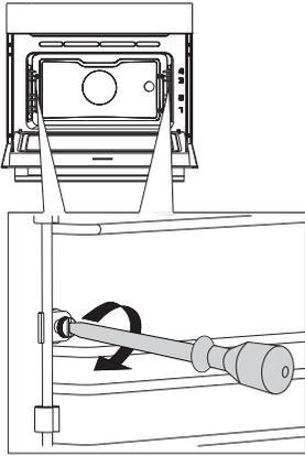
**1** Undo the screw. Use a screwdriver.
