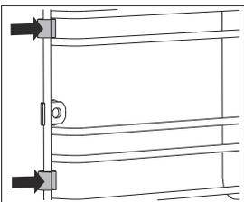
Take care not to lose the spacers fitted on the wire guides. Replace the spacers after cleaning; otherwise, sparks may appear.
