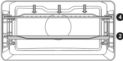
When grilling food, the upper heater and the grill heater fitted on the ceiling of the oven cavity will operate.
