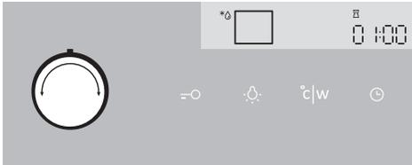
**1** Turn the COOKING SYSTEM SELECTOR KNOB to defrosting. The icon and the program A1 will flash on the display unit (choose between five programs - see table below).
