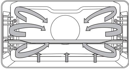
The bottom heater, the round heater, and the hot air fan will operate. Suitable for baking pizzas, apple pies, and fruitcakes.
