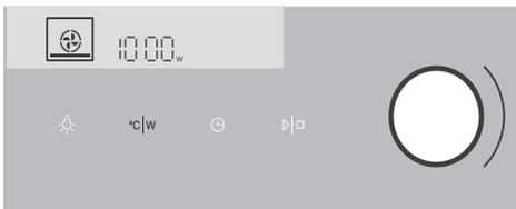
**3** Touch the TEMPERATURE KEY twice to set the power. Power in watts (W) will appear on the display. Rotate the SETTINGS KNOB (-/+ ) and set the power.
