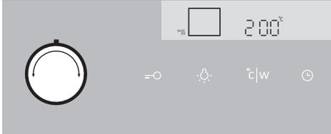
Turn the COOKING SYSTEM SELECTOR KNOB to rapid preheating. PRESET TEMPERATURE will be displayed. This temperature setting can be adjusted.
