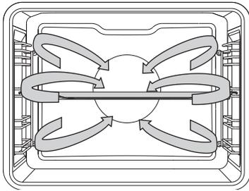
Round heater and the fan will operate. The fan installed in the back wall of the oven cavity makes sure the hot air constantly circulates around the roast or pastry.
