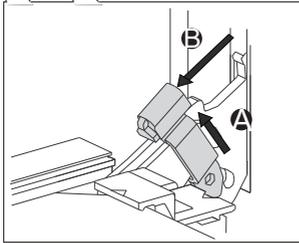
**2** Slightly lift the hinge retainers and pull the door towards you.
