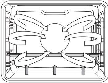
This is used for baking leavened but low-rising pastry and for preserving fruit and vegetables. Use the second guide from the bottom and a rather shallow baking tray to allow the hot air to circulate across the upper side of the dish.
