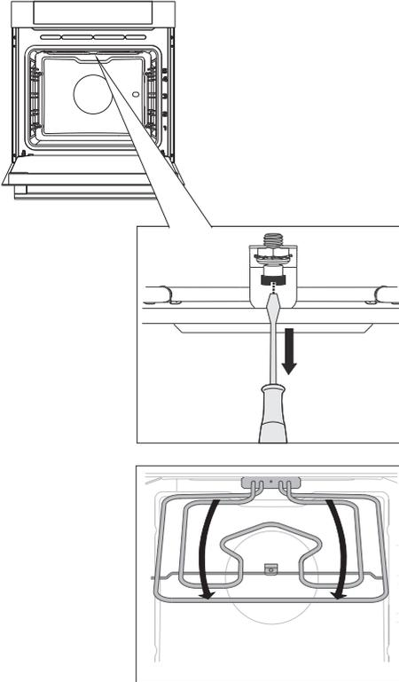
**1** To remove the heater, undo the screw located at the front of the oven cavity ceiling.
