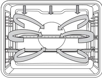
In the automatic meat cooking mode (Auto Roast), the upper heater will operate in combination with the round heater. It is used for roasting all types of meat.
