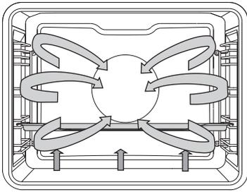
The bottom heater, the round heater, and the hot air fan will operate. Suitable for baking pizzas, apple pies, and fruitcakes.
