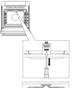
**1** To remove the heater, undo the screw located at the front of the oven cavity ceiling.
