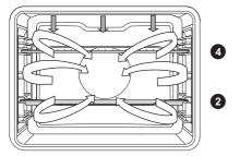
In this operating mode, the grill heater and the fan operate simultaneously. Suitable for grilling meat, fish, and vegetables.
