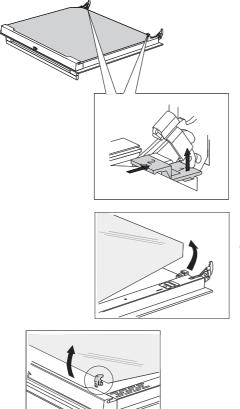
**1** Slightly lift the supports on the left and right side of the door (marking 1 on the support) and pull them away from the glass pane (marking 2 on the support).
