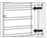
**2** Remove the guides from the holes in the back wall.
