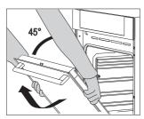
Slowly close the door to a 45-degree 3 Slowly close the door and angle (relative to the position of the fully closed door); then, lift the door and pull it out
