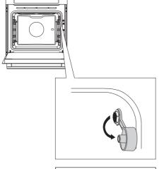
Remove the metal cap (the socket is in the front upper corner of the oven right wall).
