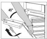
3 Slowly close the door to 2 angle (relative to the position of the Slowly close the door to a 45-degree fully closed door); then, lift the door and pull it out
