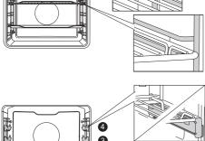
With telescopic extendible guides, first pull out the guides of one level and place the grid or the baking tray onto them. Then, push them in with your hand as far as they will ao.
