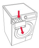
To remove the dispenser tray from the housing, press the small lever.
