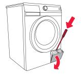
Open the filter lid using flat screwdriver or similar tool.
