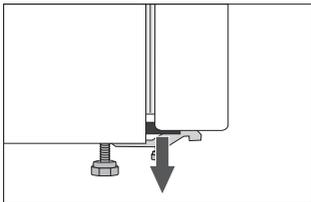
Spacers are fitted on the corners of the doors. Remove them and insert the supplied plugs into their slots (only in some models).
