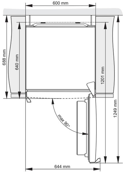
**Note:** When placing the appliances side by side, the anti-dew (anti-condensation) set has to be purchased and installed!
