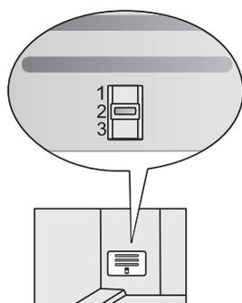
The flap is located in the fruit and vegetable bin. As a factory setting, it is in position 2. If it is not possible to reach the right temperature by adjusting the settings with the knob **A**, then set the flap as described in the section »Troubleshooting«.
