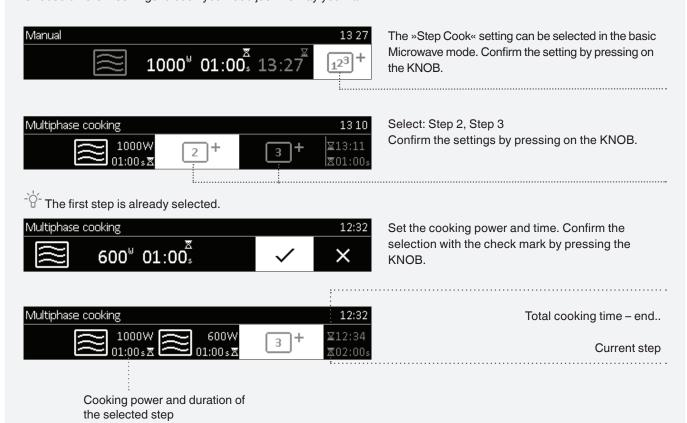
Touch the START symbol to turn on the oven. The oven starts operating immediately, with the settings defined in Step 1. (A strip at the bottom of the display indicates the cooking step currently in progress.) After the set cooking time elapses, Step 2 and then Step 3 are activated, if specified.
