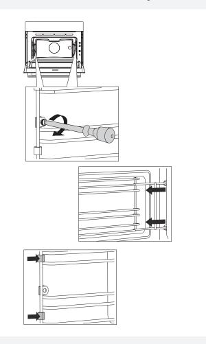
■ Undo the screw. Use a screwdriver.
