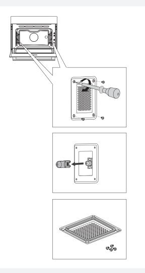
Indo the four screws on the cover. Remove the cover and the glass.
