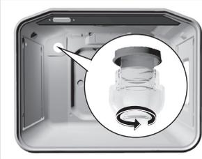
**The oven lamp base and socket are under voltage. There is a risk of electric shock!**
