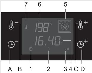
After the end of cooking process, rotate the selector knob to the “zero” position. This will also interrupt and delete all timer functions (see the section “Setting the timer functions”); the timer will switch to time of day / clock display.
