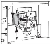
**N.B.! If the brewing unit is difficult to insert, you must first adapt it to the right dimensions by pressing it forcefully from the bottom and top.**
