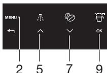
2. Press the touch key ‘MENU’ (2) and press the scroll touch keys (5 and 7) until the menu option “WATER HARDNESS” appears. Confirm the menu option with the touch key ‘OK’ (9).
