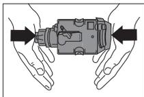
7. Once inserted, make sure the two red buttons have snapped back out, otherwise the service door cannot be closed.
