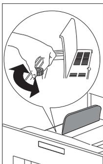
**Only change the grind level during the milling process. Otherwise, the coffee machine may be damaged.**
