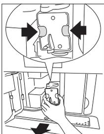
**Clean the brewing unit under running tap water without using detergent. Never clean the brewing unit in the dishwasher.**
