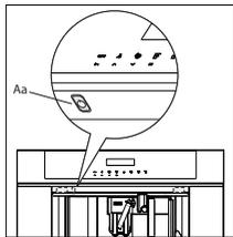
Before performing any cleaning operations, the machine must be turned off by pressing the main switch (A) and unplugged from the mains power supply. Never immerse the coffee maker in water.
