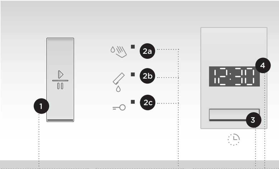
**1** **START/ PAUSE** key, use this key to start or stop the program. When selected, the signal light on the key will flash. When the program has started it will be lit continuously.
