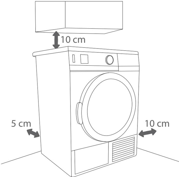
Ventilation slots and the opening on the front and rear side should always be kept free.
