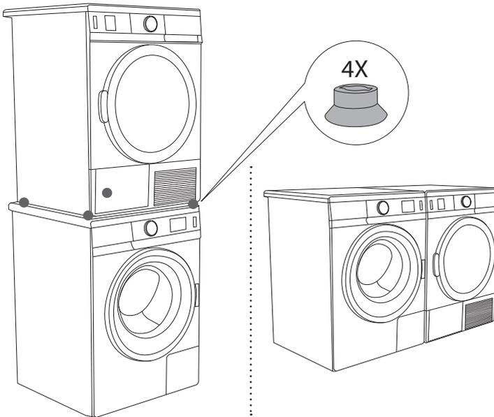
Positioning the appliance on top of the washing machine by using the vacuum feet or side by side.
