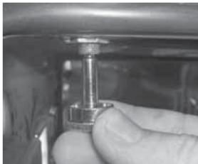
Remove the cover and insert the plug of the probe all the way (you will hear a slight confirming click).
