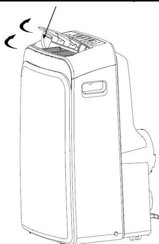
The louver can be adjusted automatically.
