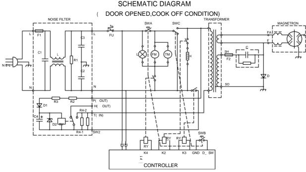
SWA: PRIMARY INTERLOCK SWITCH SWB: SECONDARY INTERLOCK SWITCH
