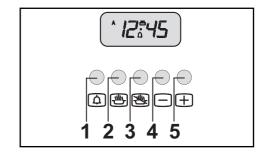
Semi-automatic working order (setting end of cooking from 0,01 to 23,59 = hh,mm)
