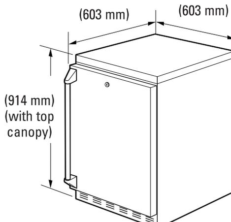
When building in the Outdoor/Indoor refrigerator, be sure to allow for a full door swing so you have full access to the pull-out full extension drawers.
