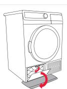
Place an absorbent cloth on the floor in front of the dryer.
