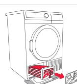
Remove the closing lid. Turn the condenser handle upwards and use the handle to pull the condenser out.
