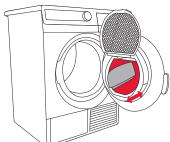
Scrape the filter cover to remove the layer of lint and threads.
