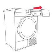
Remove the condensate tank from the dryer,
