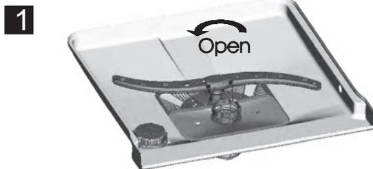
Step 1: Turn the filter in anti-clockwise direction,
