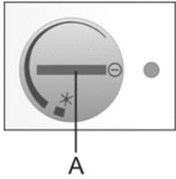
Rotate the **A** knob back to the position in which the arrow is aligned with the symbol
