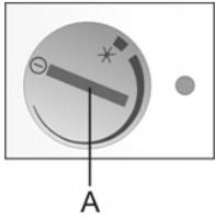
Rotate the thermostat knob **A** clockwise towards the thicker end of the sign.
