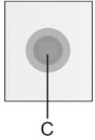
Signal light **C** will flash when the temperature in the freezer rises to a level that is too high, and goes off when the temperature drops back to a level that no longer represents food spoilage hazard (see section »Troubleshooting«).
