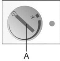
Recommended setting for the thermostat knob **A** is half way between the **thinner and the thicker** end of the sign.
