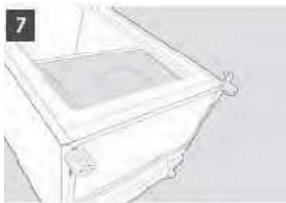
Remove bottom bracket using an 8 mm socket or spanner.
