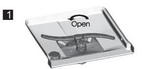
Step 1: Turn the filter in anti-clockwise direction,
