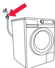
**1** Remove the net filter from the inlet hose.
