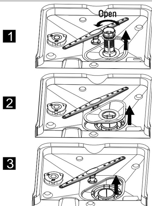
Step 1: Turn the filter in anti-clockwise direction, then lift it up.
