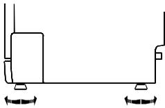
Once the appliance is positioned for levelling, the height of the dishwasher may be altered via adjustment of the screwing level of the feet. In any case, the appliance should not be inclined more than 2°.
