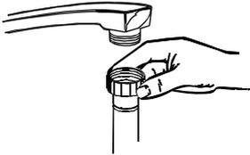
Connect the cold water supply hose to a threaded 3/4 (inch) connector and make sure that it is fastened tightly in place. If the water pipes are new or have not been used for an extended period of time, let the water run to make sure that the water is clear. This precaution is needed to avoid the risk of the water inlet to be blocked and damage the appliance.
