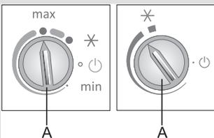
Rotate the thermostat knob **A** clockwise towards the thicker end of the sign.
