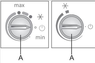
Rotate the **A** knob back to the position in which the arrow is aligned with the symbol
