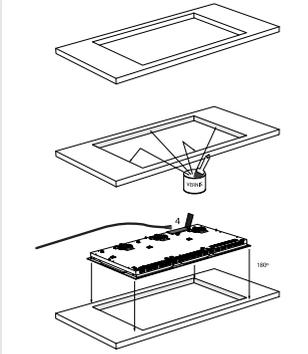
Check that the cabinet and the cut-out meet the dimension and ventilation requirement
