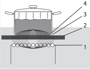
Coil (1) in the induction hob (2) generates magnetic field (3). When a pan with ferromagnetic metal bottom (4) is placed on the coil, eddy currents are generated in the pan bottom, which produce heat.
