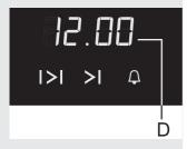
• Each time the appliance is connected to the power mains, "12.00" will flash on the display.
