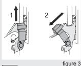
• If the appliance is fitted with the GentleClose system, slightly lift the door latches and pull them towards you.
