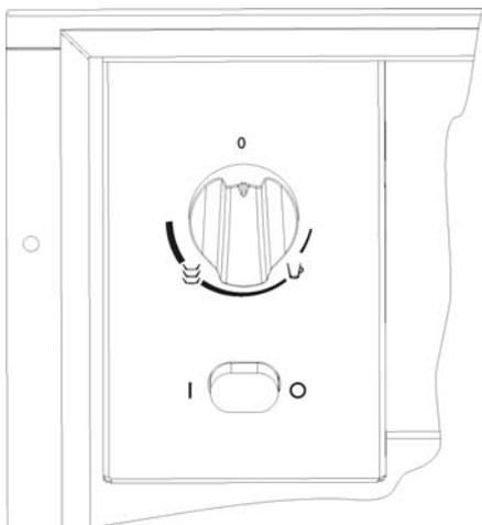
The control panel has a temperature selector and the on/off switch. The control panel is only visible when the drawer is open.
