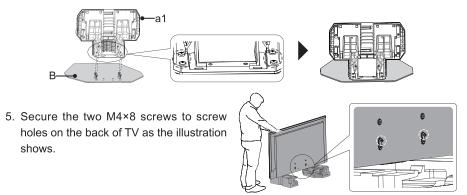
6. Hang the assembled Part a1 and Part B to the two M4×8 screws you have secured to the TV, then secure the assembled part to TV with four M5×16 screws. You can adjust the height of base stand to H1 or H2. For H1, secure screws to four hole 1. For H2, secure screws to four hole 2.
