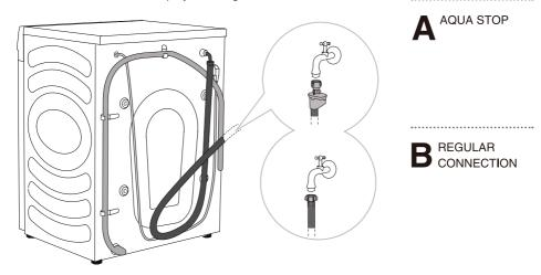
'ŷ' For normal washing machine operation, the pressure in the water mains should be between 0.1-1 MPa (1-10 bar; 1-10 kp/cm<sup>2</sup>; 10-100 N/cm<sup>2</sup>). Minimum dynamic water pressure can be determined by measuring the water flow. In 15 seconds, 3 litres of water should flow from a fully open tap.
