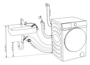
Discharge hose end may be placed over a sink or a bathtub. B Use a string fed through the opening in the elbow support to attach the hose and prevent it from slipping to the floor.
