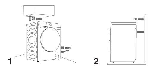
'Ġ' The washing machine may not be in contact with a wall or adjacent furniture. For optimum washing machine operation, we recommend observing the clearances from the walls as indicated in the figure.
