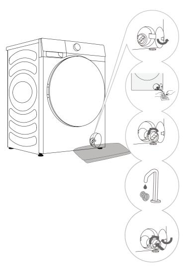
Open the pump filter cap (Press the door cover and automatically pop open).
