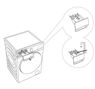
To remove the detergent compartment from the housing, press the small tab.
