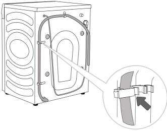
The discharge hose has to be attached and affixed to the pin on the back of the washing machine, as shown in the figure.
