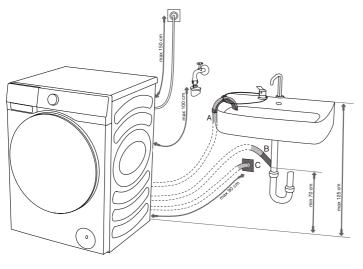
Discharge hose can also be attached to a wall drain with a trap; such trap should be properly installed to allow cleaning.
