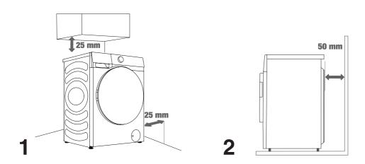
$\dot{\nabla}$  The washing machine may not be in contact with a wall or adjacent furniture. For optimum washing machine operation, we recommend observing the clearances from the walls as indicated in the figure.
