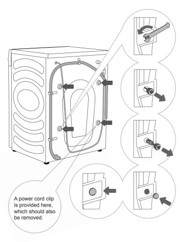
Move aside the hoses and use a fitting spanner to undo the 4 screws on the back of the appliance by turning them counter clockwise, as indicated by the arrow. Undo them by approximately 30 mm (not completely).
