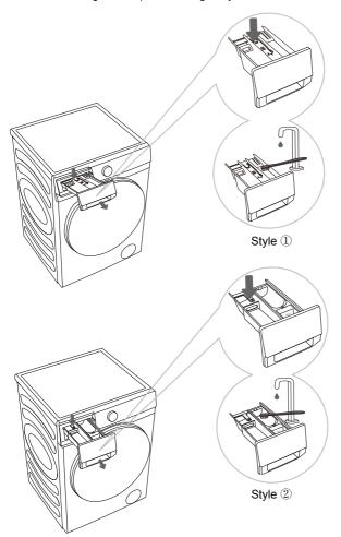
To remove the detergent compartment from the housing, press the small tab.
