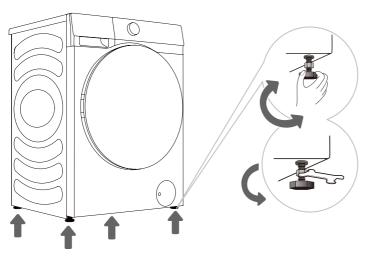
Rotate the adjustable feet to level the washing machine lengthwise and crosswise. The feet allow levelling by +/- 2 cm.
