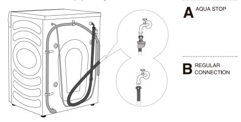
'ŷ' For normal washing machine operation, the pressure in the water mains should be between 0.1–1 MPa (1-10 bar; 1–10 kp/cm²; 10–100 N/cm²). Minimum dynamic water pressure can be determined by measuring the water flow. In 15 seconds, 3 litres of water should flow from a fully open tap.
