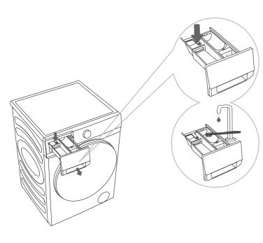
To remove the detergent compartment from the housing, press the small tab.
