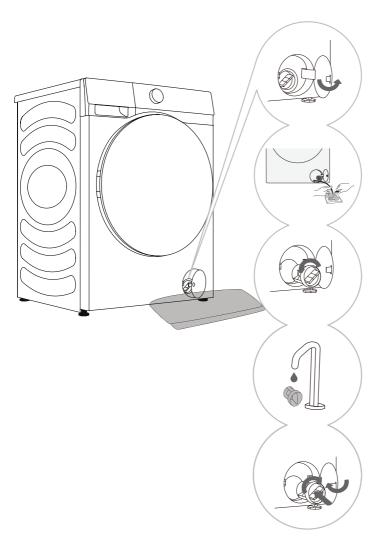
1 Open the pump filter cap (Press the door cover and automatically pop open).
