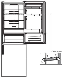
2. Remove part ①, loose part ② from the top right side of refrigerator.
