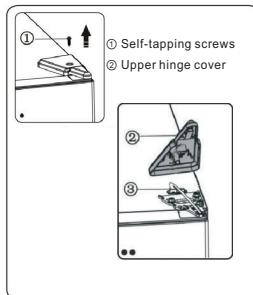
3. Remove screws ① and hinge
