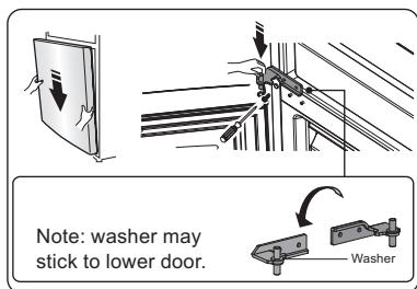
15. Move the upper door to an appropriate position, and then fix
