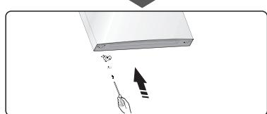
10. Change screw hole covers on middle cover plate from left to right (as shown in figure below).
