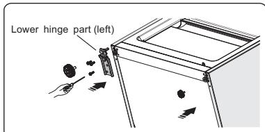
14. Slot the lower door onto the bottom hinge pin and hold in position. Turn the middle hinge by 180°, change the washer on the axis to the lower side, adjust the middle hinge to the appropriate position and then install it ensuring the lower door in secured place.
