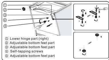
12. Remove part ③ from the lower hinge pin, loose out the lower hinge pin, change it to the reverse hole site, and then tighten into position, then install part ③ on the lower hinge pin.
