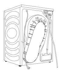
Remove discharge hose from the machine and hang it on the back.
