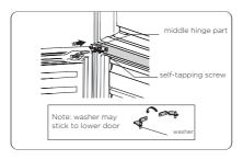
14. Transfer the upper door to the appropriate position. Secure the door's level, make the middle hinge axis into the lower hole of the upper door.
