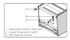
9. Remove part (1) from the lower hinge part(right), loose out the lower hinge pin, change it to the reverse hole site, and then tighten into position, then install part (1) on the lower hinge pin.
