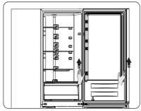
4.Loose screw (3) and take down part (2) and part (1), Install replacement door stopper-left (4) (provided in the plastic bag) and part (2) (stop block) to the left side with screw (3). Keep part (1) with the appliance for future reference.
