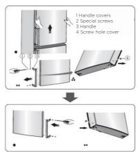
**Warning!** When changing the side at which the door opens, the appliance must not be connected to the mains. Remove plug from the mains beforehand.
