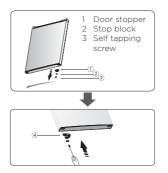
7. Change screw hole covers on middle cover plate from left to right (as shown in figure below).
