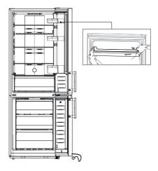
2. Remove part (1), then take down part (2) from the top right side of refrigerator. Unscrew screws (3) by a 8 mm socket driver or a spanner, and remove hinge (4). Please hold upper door by hand when installing. Use a putty knife or thin-blade screwdriver to lever part (5) which is at the top left corner of the refrigerator.
