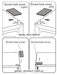
6. When the refrigerator with a display on door, remove part ① from the top left side of upper cover and take out part ② . Then remove part ③ and put part ④ into the top right side of upper cover. Refer to above operation, install part ③ and part ④ on to the top left side of upper cover.Install part ① of the top right side of upper cover. When the refrigerator without a display on door, skip this step.
