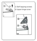
3.Remove screws ① and hinge ②.When the refrigerator with display on door, you need to pass connector ③ through the hole of hinge②.(Please hold upper door by hand when installing).
