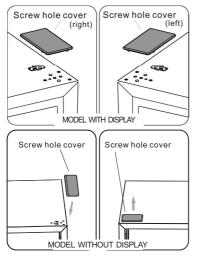
6.When the refrigerator with a display on door, remove part ① from the top left side of upper cover and take out part ② . Then remove part ③ and put part ④ into the top right side of upper cover. Refer to above operation, install part ③ and part ④ on to the top left side of upper cover.Install part ① of the top right side of upper cover. When the refrigerator without a display on door, skip this step.
