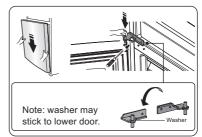
15. Move the upper door to an appropriate position, and then fix
