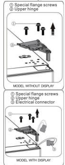
4. Remove the upper door from the middle hinge by carefully lifting the door straight up. Then place the upper door on a smooth surface with its upper cover upwards.
