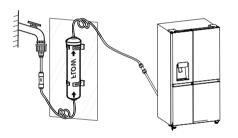
• The water lines should not be pressed by heavy things and should not bend too much.
