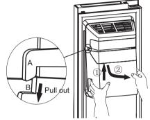
When you put it back, please make sure the two side(B&B') of Ice Bucket is wedged into the buckles(A&A').
