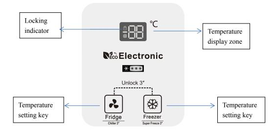
**NOTE:** High temperature setting will accelerate food waste. Note: This figure is only a schematic diagram, so please refer to the physical object for details.
