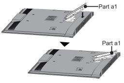
4. Secure Part a1 with 4 screws (M5×12) onto the back cover of the TV.
