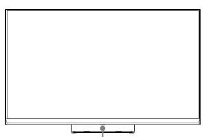
Remote sensor/Light sensor/Power indicator/Single button (Standby/Source)
