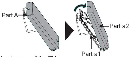
3. Put Part a1 onto the back cover of the TV.
