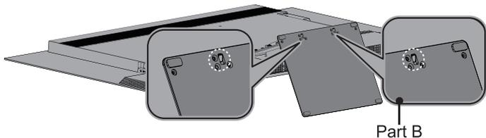
6. Then, secure Part B with 6 screws (M5×16).
