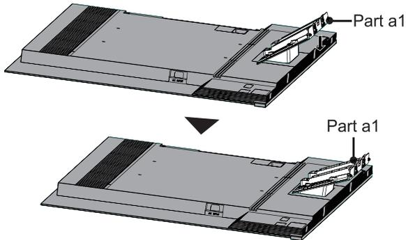
4. Secure Part a1 with 4 screws (M5×12) onto the back cover of the TV.
