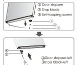
11. Change screw hole covers and screw on middle cover plate from left to right (as shown in figure below).
