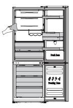
Although this appliance automatically defrosts, a layer of frost may occur on the freezer compartment's interior walls if the freezer door is opened frequently or kept open too long. If the frost is too thick, choose a time when the freezer is nearly empty and proceed as follow:
