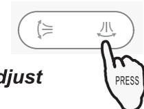
**NOTE:** If the unit doesn't have four ways airflow function, you can adjust horizontal airflow by yourself.
