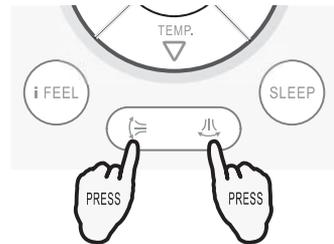
The direction of airflow can be also adjusted to your own requirement by pressing the " " button of the remote controller.
